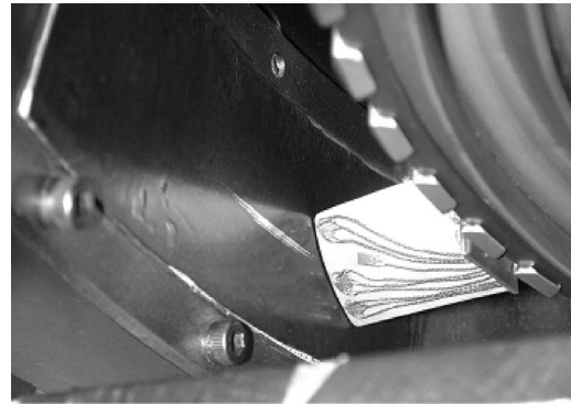
Fig. 12 Blade and casing after very light rub
